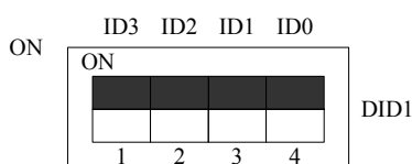
The above chart shows "1111", so it means that the physical ID is 15.
